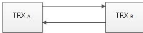
Figure 1.1: A point to point communication link.
