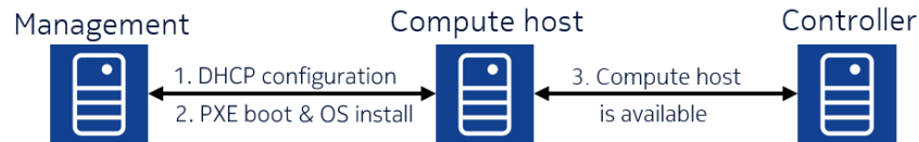
Figure 6.1: When OpenStack cloud is expanded, new compute hosts can be installed by using network boot.
