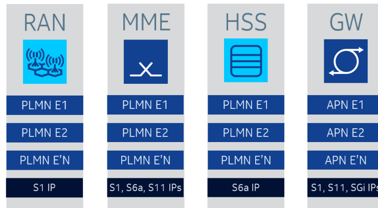
Figure 5.9: Typically, PLMNs and APNs can be used for logical division and elements need IP connectivity, too. In real life, there is a huge number of parameters that have to be set.
