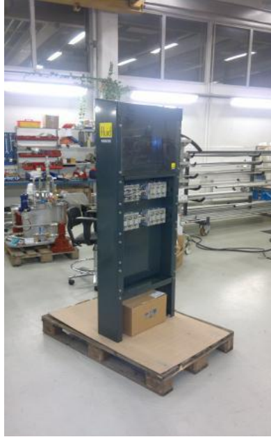
Figure 1.1. Oil lubrication measurement station from Fluid House.
