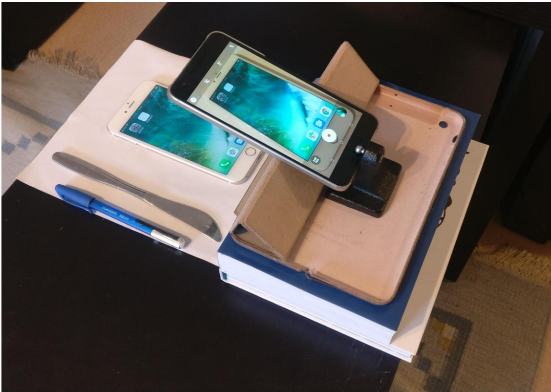
Figure 1. The high-speed camera video recording setup with a Nexus 6P acting as a camera.
