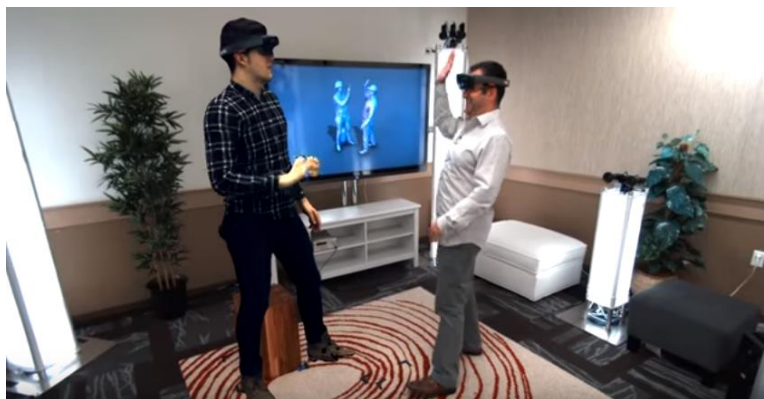
Figure 11: Screenshot of video from Microsoft Research Holoportation project. The man standing on the left side is virtual. (Cutler, Fowers, and Chang, 2016)
