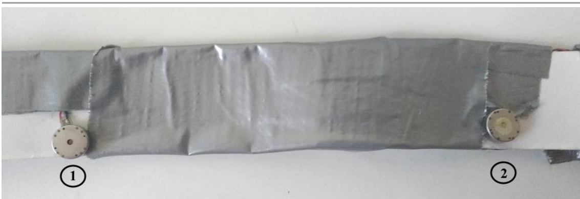
Figure 7. Two vibrotactile actuators fixed into a headband
