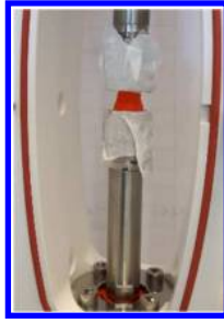
Scheme 4: The hydrogel sample (red) placed between the tips of Bose Compression Testing Machine.
