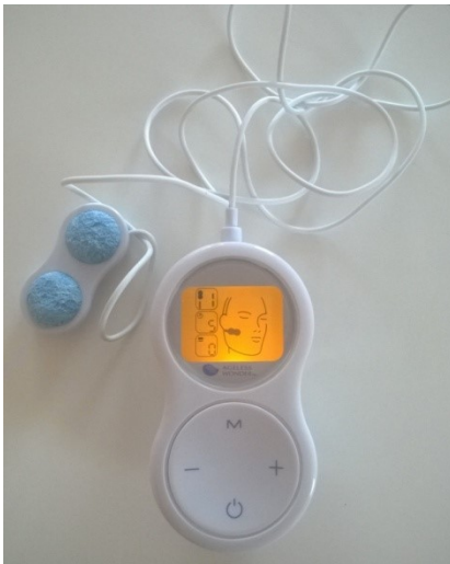
Figure 4. Ageless Wonder™: a control panel and a wand with two electrodes (blue sponges) connected with a wire.
