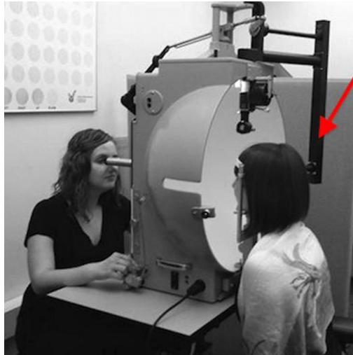
Figure 6. The Goldmann perimeter in use. The patient gazes into the hemispherical bowl while the examiner displays stimuli on it's surface. [Fortenbaugh et al., 2012]
