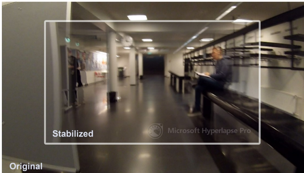
Figure 9. The stabilized image superimposed on the original image that shows the field of view difference.
