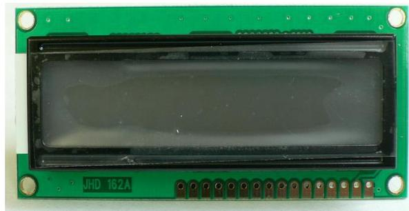
Figura 10: display 16X2 caracteres LCD-016M002B
