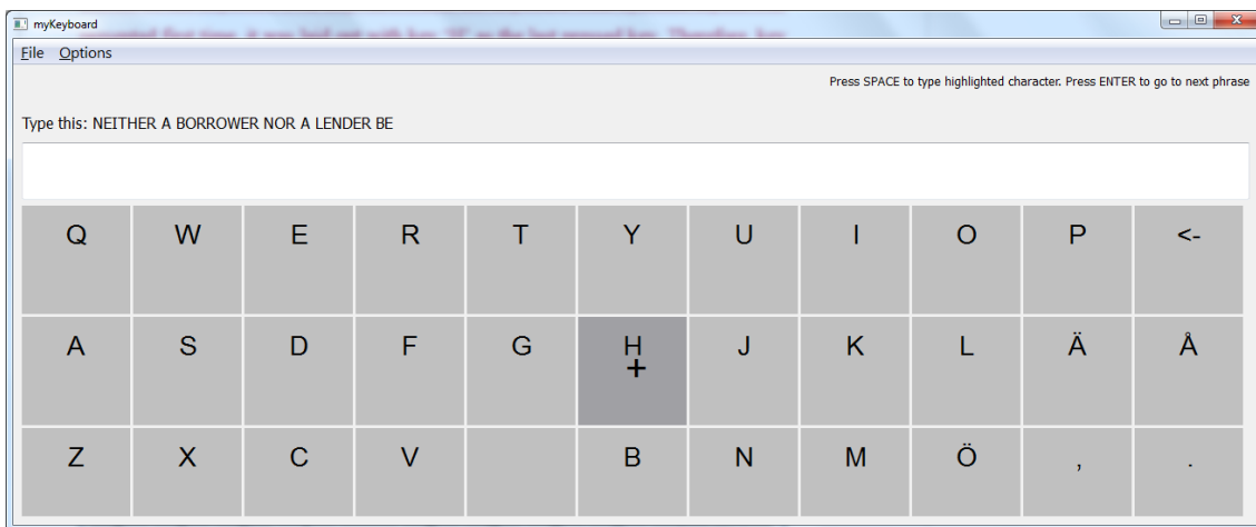
Figure 13. Text entry prototype “myKeyboard” with the static keyboard option selected.
