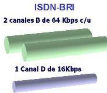
Figura 2-28 Basic Rate Interface
