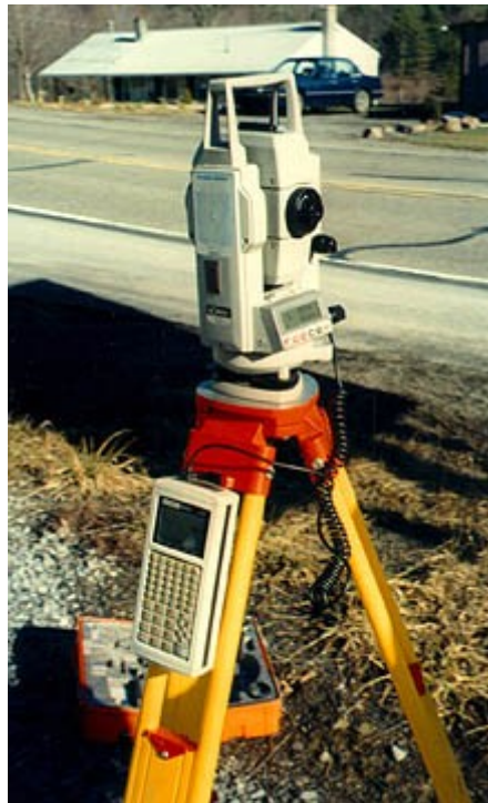
Figure 3 A total station mounted on a tripod [35]
