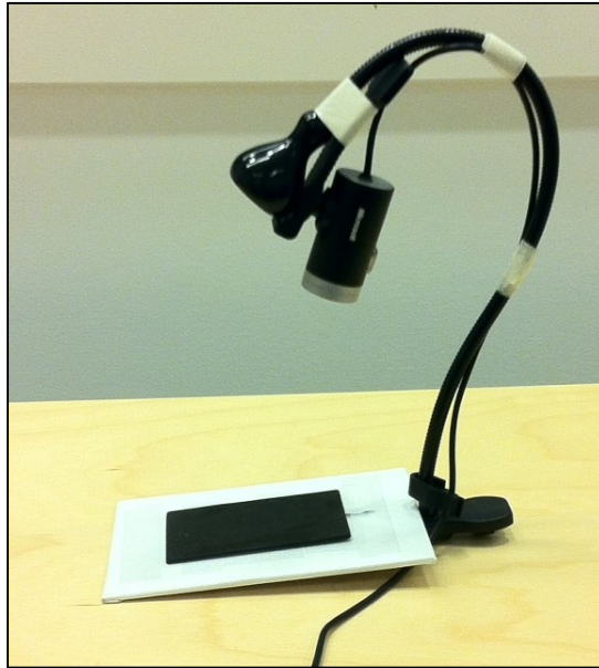
Figure 33. Usability testing rig used in the experiment, consisting of a web camera attached to a gooseneck lamp, mounted on a piece of cardboard that had a rubber adhesive pad.
