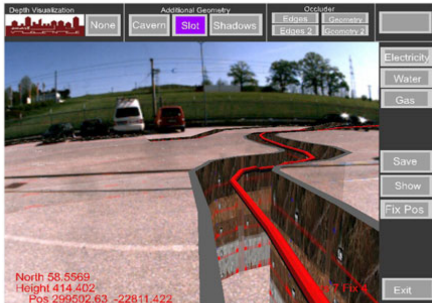
Figure 10: Smart Vidente augmented reality visualization showing underground features overlaid on a view of the real world on ground level [Schall et al., 2013]
