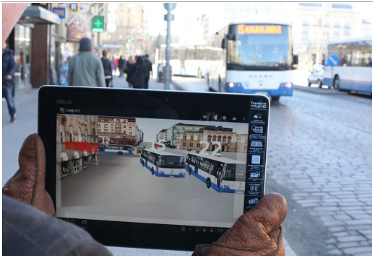
Figure 9: 3D visualization (AV) of real time tracked public transportation, displaying the bus numbers on top of the virtual vehicles. A red occluded vehicle is also shown on the left of the device's screen [Nurminen et al., 2014]
