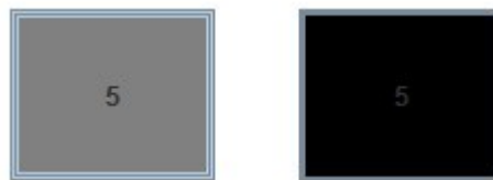
Fig. 18. Button states for the hover and mousepress events when the screentap input method is being used. On the left, visual feedback when cursor is hovering on the button. On the right, visual feedback when the button is clicked.
