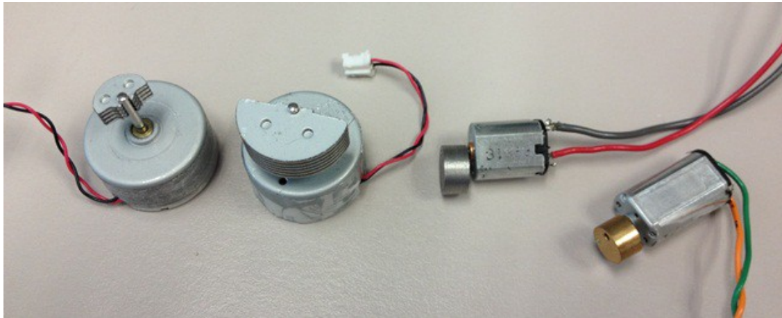
Fig. 6. Eccentric rotating mass vibration motors. On the left, Xbox 360 vibration motors and on the right, motors used in vibrating toys. [Image source: http://openxplatform.com/projects/shift-knob.html ]
