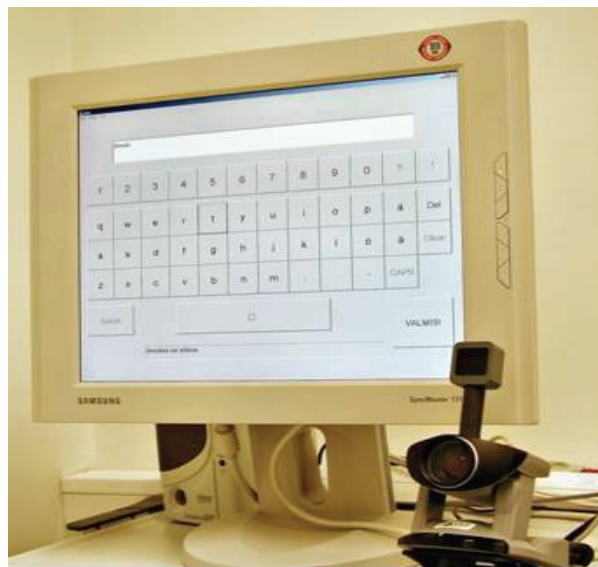
Figure 2.3 An on-screen QWERTY keyboard and an eye tracking device. The eye tracker follows the user's gaze and the computer analyzes the gaze behavior. The pointed character is shown highlighted on the keyboard layout [Majaranta et al., 2006].
