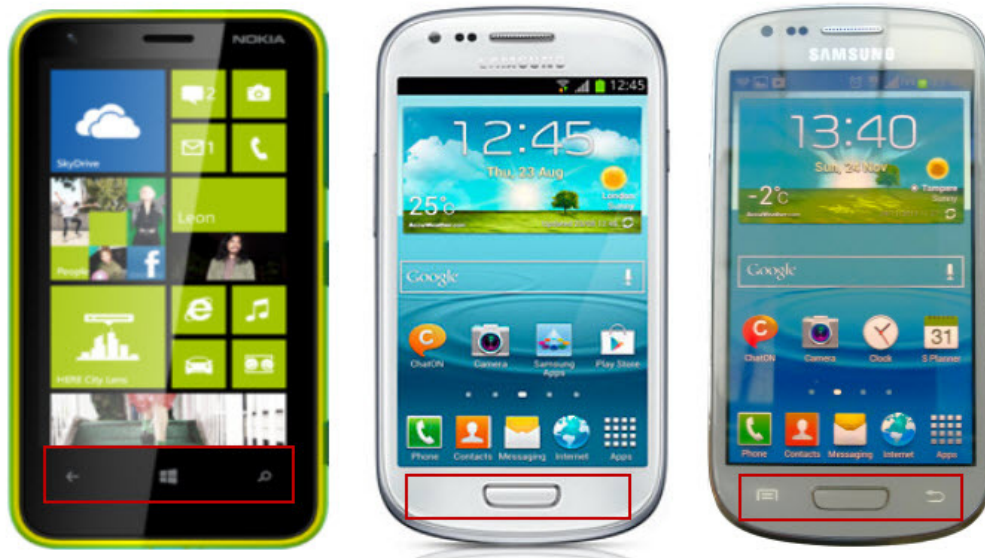
Figure 24. Back, Windows (home) and search buttons of Windows Phone on the left. In the middle Android when the menu and back buttons are not active, and on the right menu and back buttons are activated [Nokia, 2013] [Samsung, 2013].
