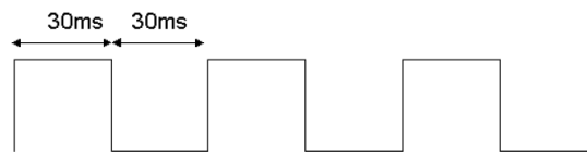
Figure 12 ON and OFF vibration pulse to phone [Brown and Kaaresoja, 2006]
