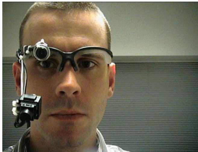
Figure 5 Low cost head worn gaze tracker from the OpenEyes project [Li et al., 2006]
