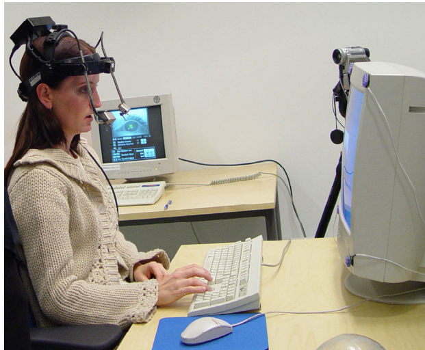
Figure 4: The test set-up and the eye tracker
