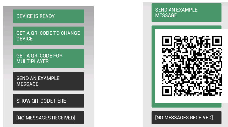
Image 1: PhoneGap application running on Android Emulator. QR code is used to pair devices.
