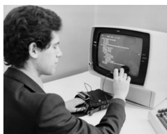
Figure 10. Vibrotactile output techniques – Optacon I and II [ASPHI, Web site; Telesensory Corporation, Web site].
