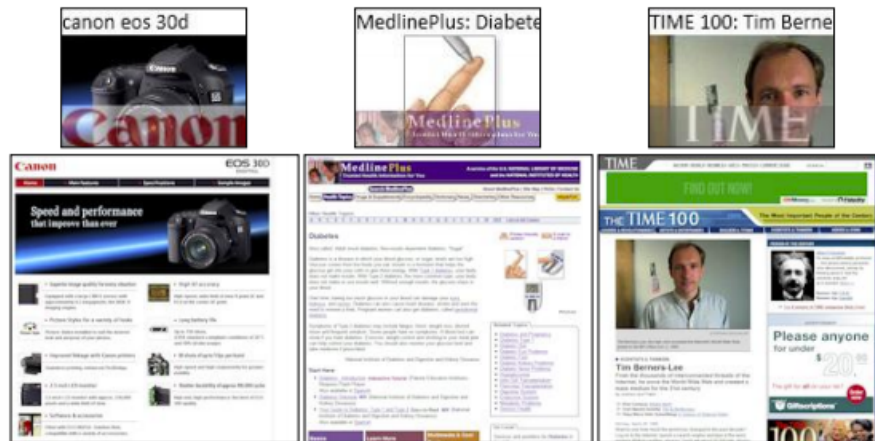
Figure 11. Visual snippets, consisting of logo, salient content image, and title, alongside the full Web pages (Teevan et al., 2009, Figure 3, © 2009 Association for Computing Machinery, Inc.).
