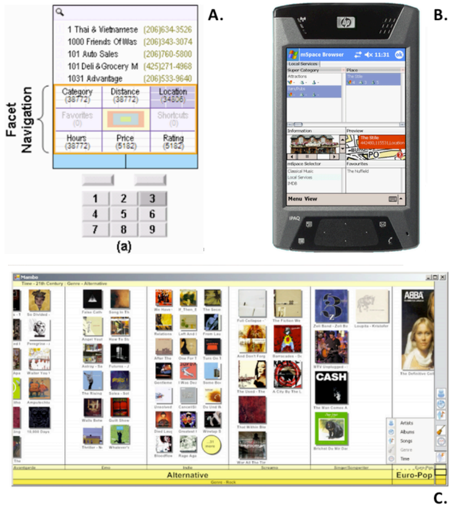
Figure 19. Approaches to faceted search and browsing: a) The FaThumb interface (Karlson et al., 2006, Figure 2a, © 2006 Association for Computing Machinery, Inc.), and b) the mSpace Mobile interface (courtesy of Max L. Wilson), and c) the Mambo music browser interface (Dachselt & Frisch, 2007, Figure 1, © 2007 Association for Computing Machinery, Inc.).
