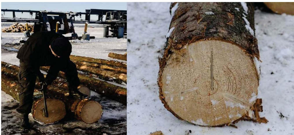
Fig. 2. Manual application of the transponder into the log end.
