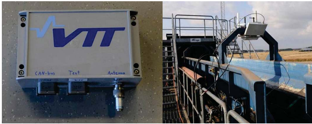
Fig. 3. Developed RFID reader prototype for the harvester and a test reader set-up at a saw mill.
