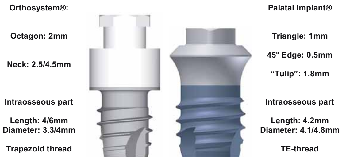
Fig. 4 Construction characteristics of Straumann Orthosystem® and Palatal Implant®
