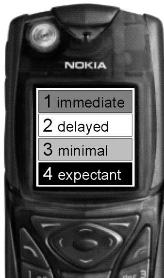
Figure 1 The triage category data entry screen in the Nokia 5140i mobile phone
