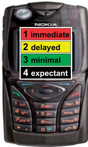
Figure 2. The triage category data entry screen in the Nokia 5140i mobile phone.
