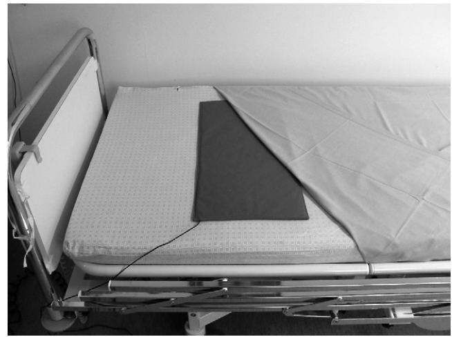
Fig. 1. Emfit movement sensor placed on an ordinary mattress below a bed-sheet.
