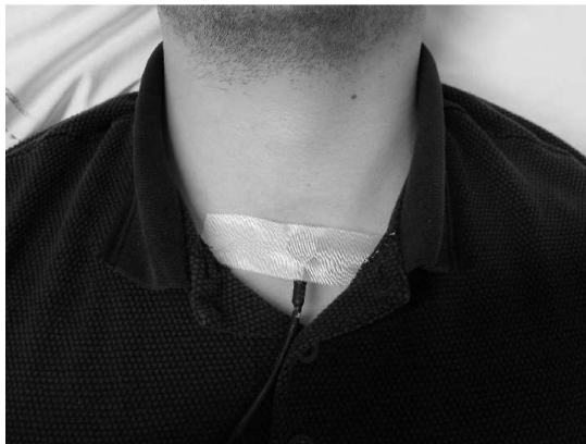
Figure 3. The microphone is attached to the jugulum in the tracheal sound recording.
