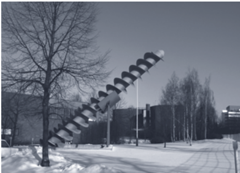
Fig. 5.4 Archimedes screw pump -- one of the most ancient water technologies still in use at Viinikanlahti wastewater treatment plant. The pictured one is no longer in use but has commemorated the 100th anniversary of the works since 1998 (Photo: T. Katko).
