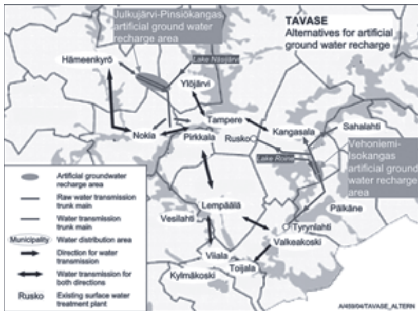
Fig. 9.4 Tavase Ltd, regional wholesale company is planning to use artificial recharge in Vehoniemi-Isokangas area in the south-eastern part of the area. Julkujärvi-Pinsiökangas area in the north-western part is planned to be taken to use later as an option.
