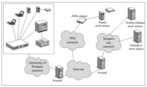
**Operating environment in Tampere.** The diagram clearly shows how the project's Net server at the University of Tampere (with the smaller, inserted figure describing the editorial set-up and the server at the university) in most cases was behind complex network connections. The main practical difficulty this caused was in updating web sites from the workstations in the two neighbourhood libraries.
