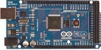
A standard rectangular blue PCB board. It features a large ATMEGA2560 microcontroller in the center, a USB Type-B port on the left, and a long edge connector on the right. The board is populated with various electronic components like capacitors and resistors. |
