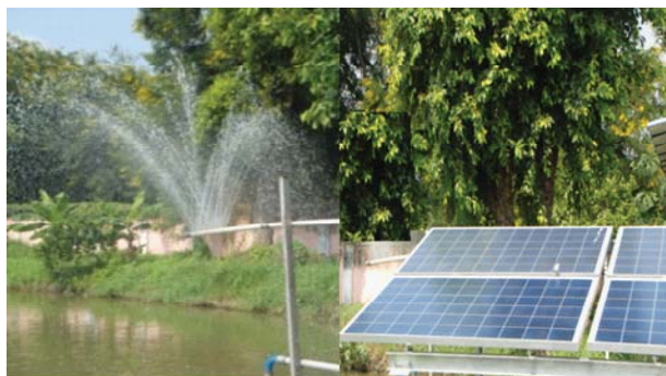
Fig. 16.7. A spray type solar aerator installed in fish pond at ICAR RCER, Patna
