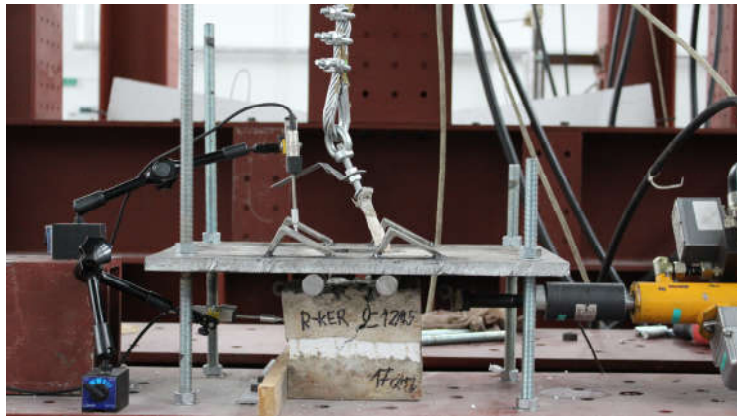
Figure 2 – The course of testing the sample anchored at an angle of 90°
