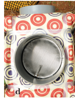
Fig 8d. A filter placed above the groove
