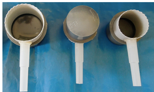
Fig. 4. Connectors of different diameter attached with hard tubular tube
