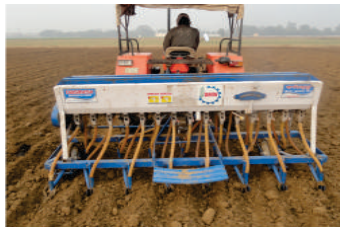
Minimum tillage sowing by seed cum fertilizer drill
