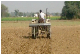
Conventional tillage sowing by single box seed drill
