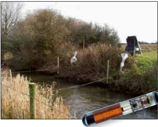
Figure 2. PIT detector installed 10 m upstream of the mouth of the side stream. The two antennas encompass the entire stream and can be seen extending above the water surface. Use of two antennas enables the direction of fish movements to be recorded. Inset on the picture is a PIT tag (actual size 23 mm).
