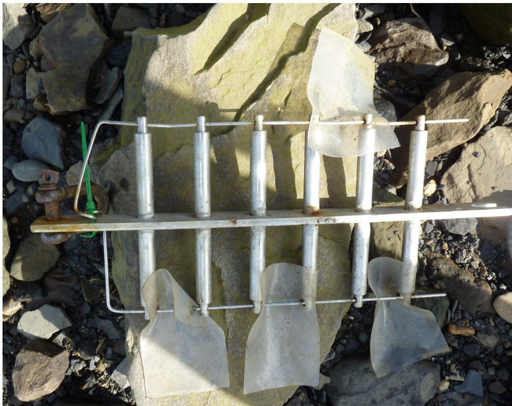
Figure 2. Retrieval of passive samplers from water after three months of exposure in the small boat harbour. Photo: Pernilla Carlsson.
