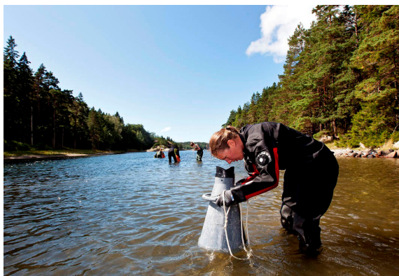
Figure 2. Sampling site at the Tjärnö area, Sweden, and application of aquascope (Photograph by Johan Wingborg, University of Gothenburg).
