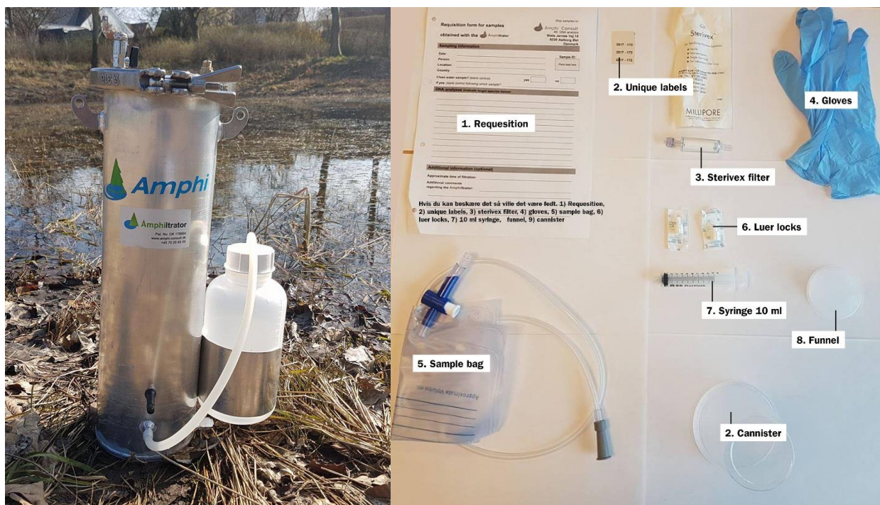
Figure 13: Amphiltrator and sample KitB.
