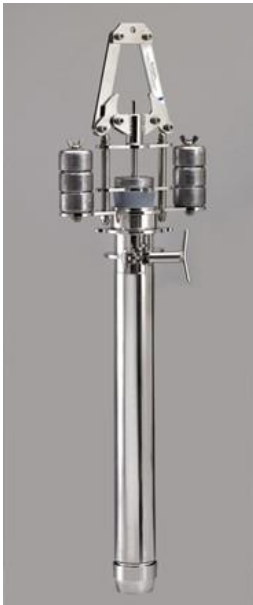
Figure 8: Kajak corer: 5.5 cm in diameter.
