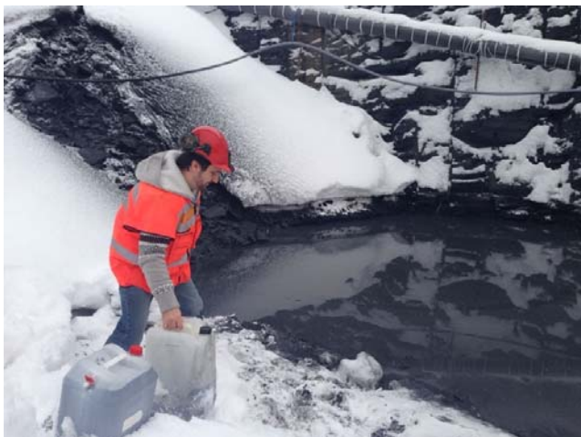
Figure 3. Sampling of tunnelling waste water from a pond collecting water pumped out from the tunnel in Gran, rv. 4.
