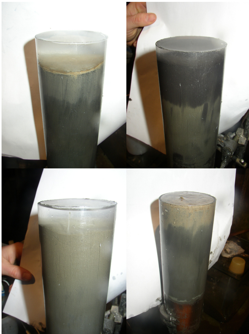
Figure 7. Core samples 05.01.07. Top left: barite cuttings (box 9), top right: ilmenite mineral (box 12), lower left: control (box 14), lower right: barite cuttings (box 16). Thickness of added layer is clearly seen in top left core
