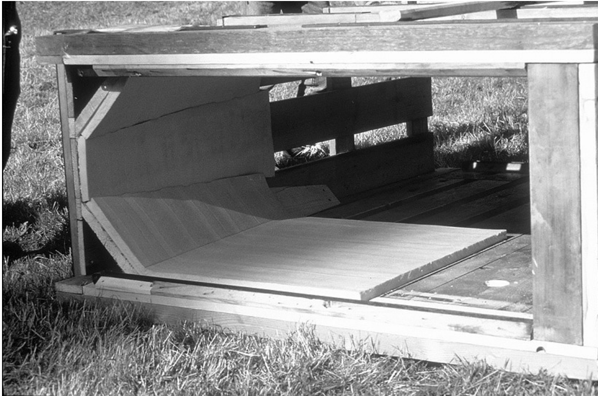
Fig. 5.10. Transport crate lying on its side. The head area of the adapted crates is reduced in order to limit the possibility of a horse turning onto its back in-flight. Additionally, the head area is lined with high-density foam to prevent injury.
