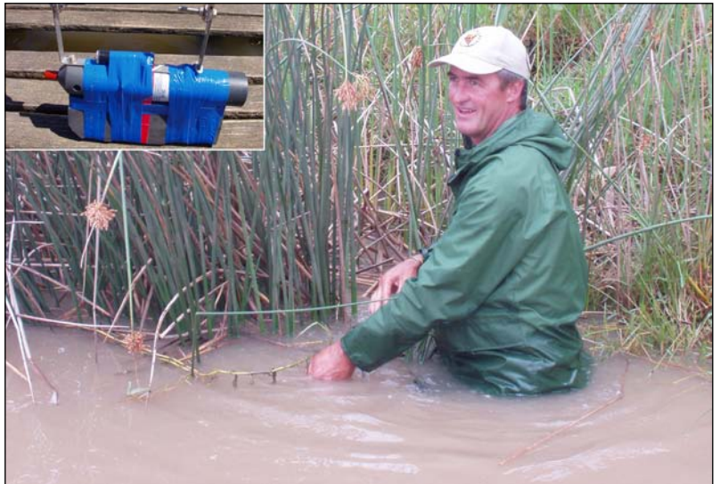
Automated data logger being placed in the upper part of the estuary.
