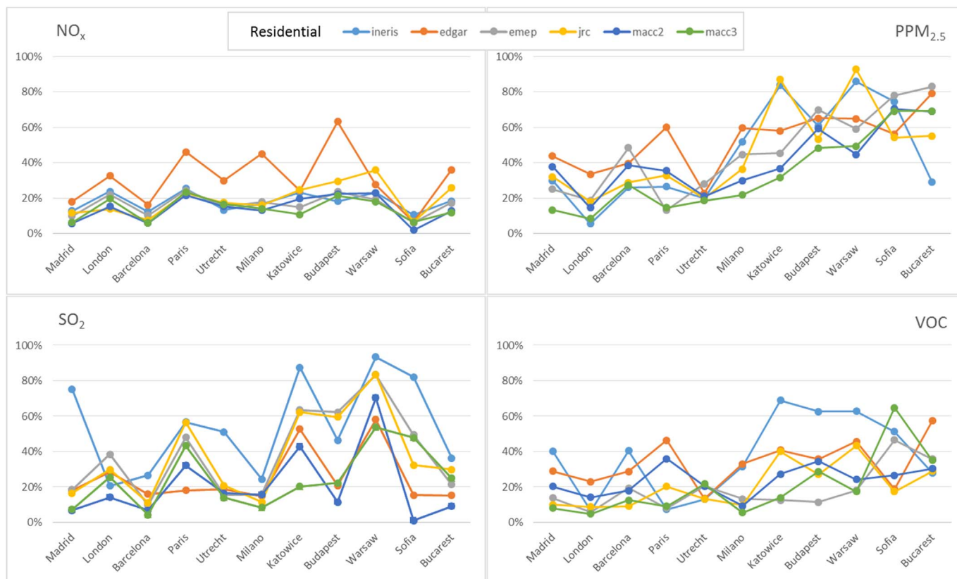
Fig. 5. Sectorial allocation. Share of the total emissions for each city coming from the SNAP02, residential combustion sector.
