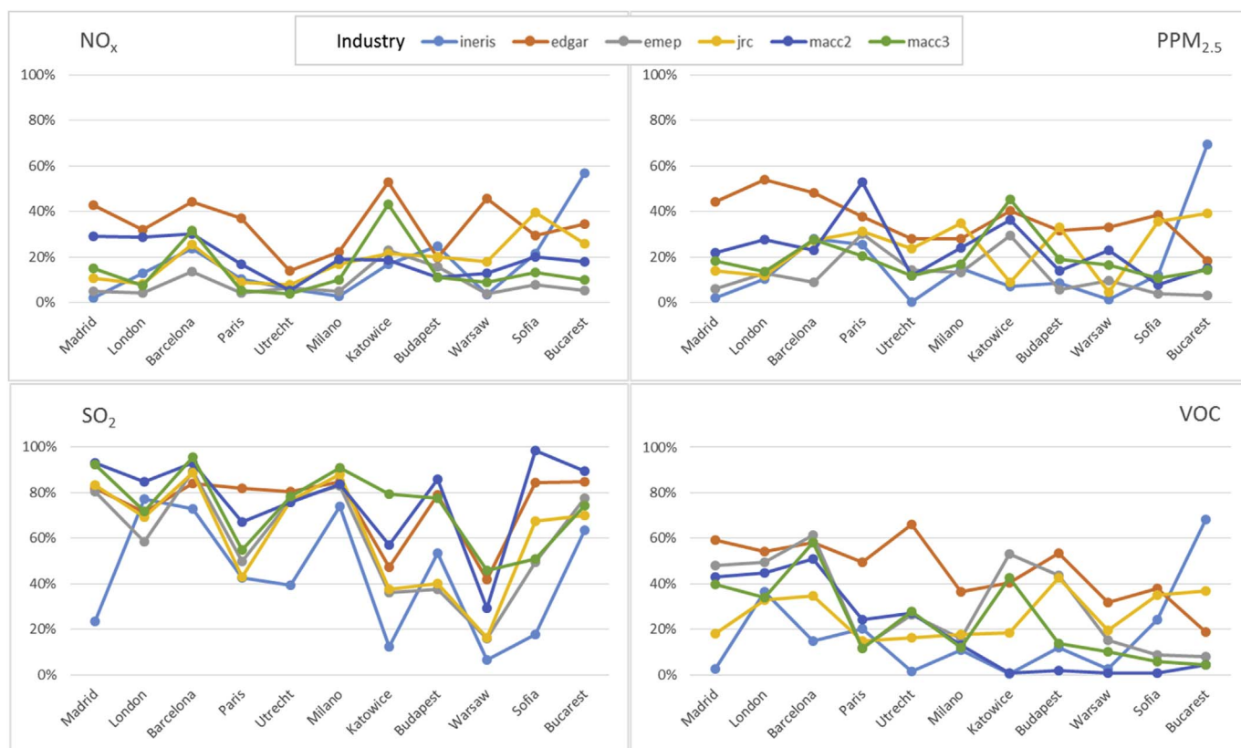
Fig. 3. Sectorial allocation. Share of the total emissions for each city coming from the Industry sector.
