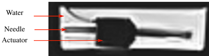
FIGURE 15: MRI IMAGE OF ACTUATOR WITH NEEDLE IMMERSSED IN WATER.
