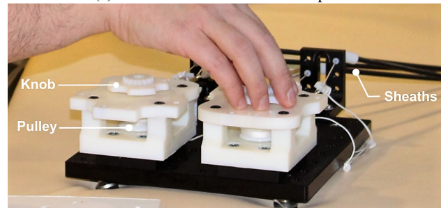
(b) Master interface for remote control of needle orientation.
