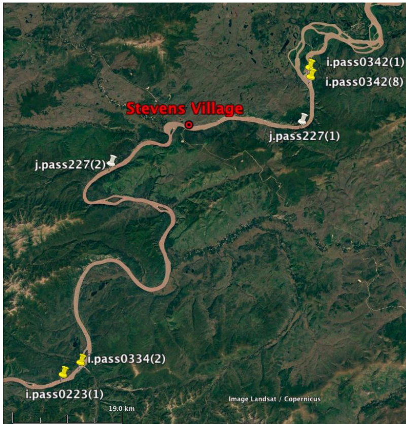
Figure 4 – Jason-2 (white pushpins) and ICESat (yellow pushpins) satellite crossing locations on the Yukon River reach near Stevens Village, Alaska. Jason-2 pass227 crosses both upstream (j.pass.227.1) and downstream (j.pass.227.2) of the USGS streamgauge site near Stevens Village (latitude 65.87 deg. W, longitude 149.72 deg. N marked by red circle.) ICESat pass 0342 (upstream), and passes 0223 and 0334 (downstream), are utilized in the study.
