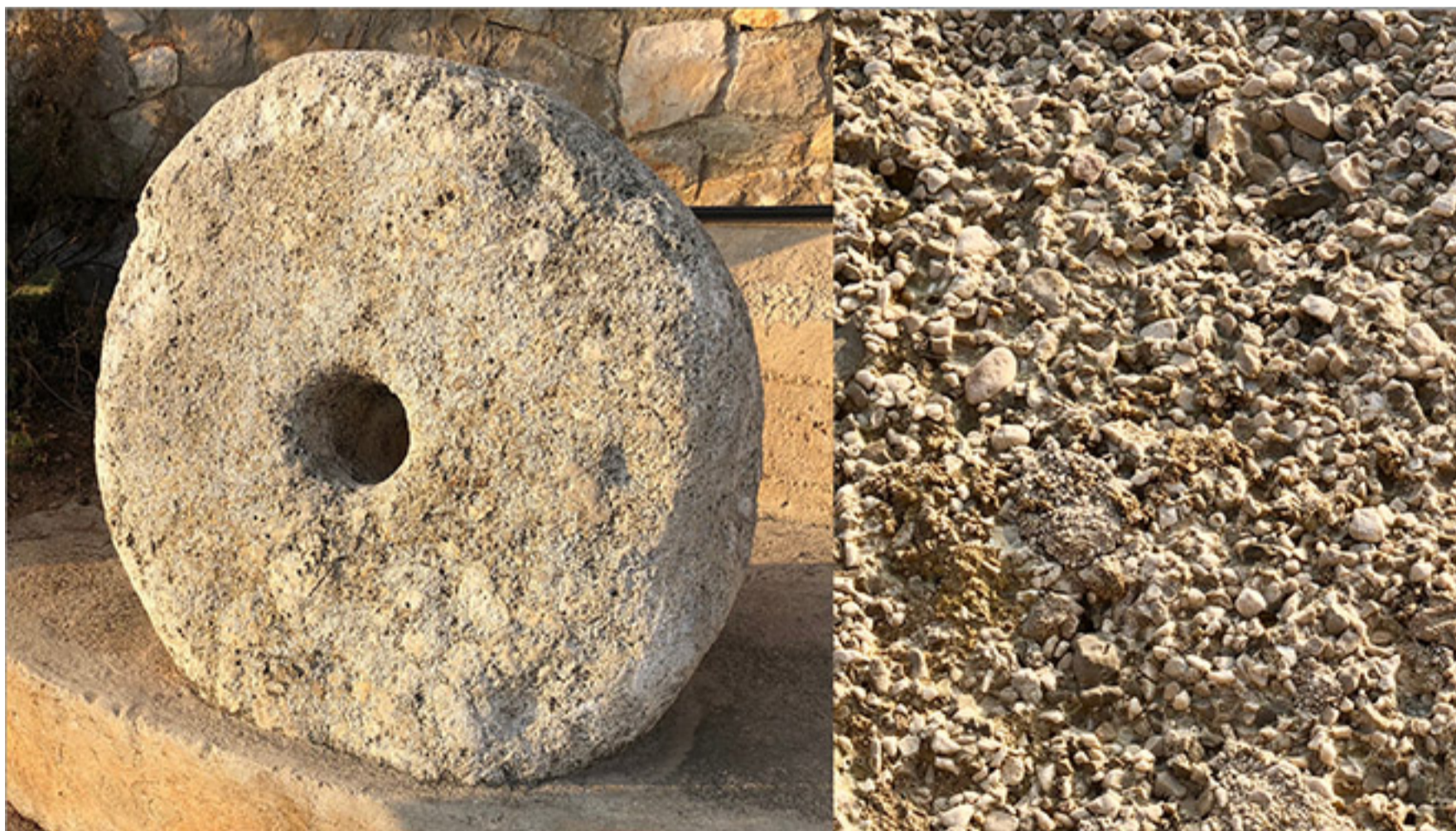
Figure 3-7: External abrasives: Example of a stone wheel of Roman era, coming from the marine quarry of Cap d'Ail (France), likely, by its heterogeneous composition, to release very abrasive silica particles. Poorly cleaned foods may retain abrasive soil residues on their surfaces, or may contain abrasive silica from poor quality stone grinders used to reduce cereals to flour prior to the introduction of industrial milling using metal devices. External and internal abrasives are the two main causes of attrition to which must be added the biocorrosion.
