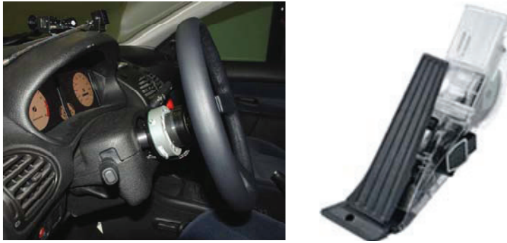
Figure 6 By wire Steering wheel and active pedal
