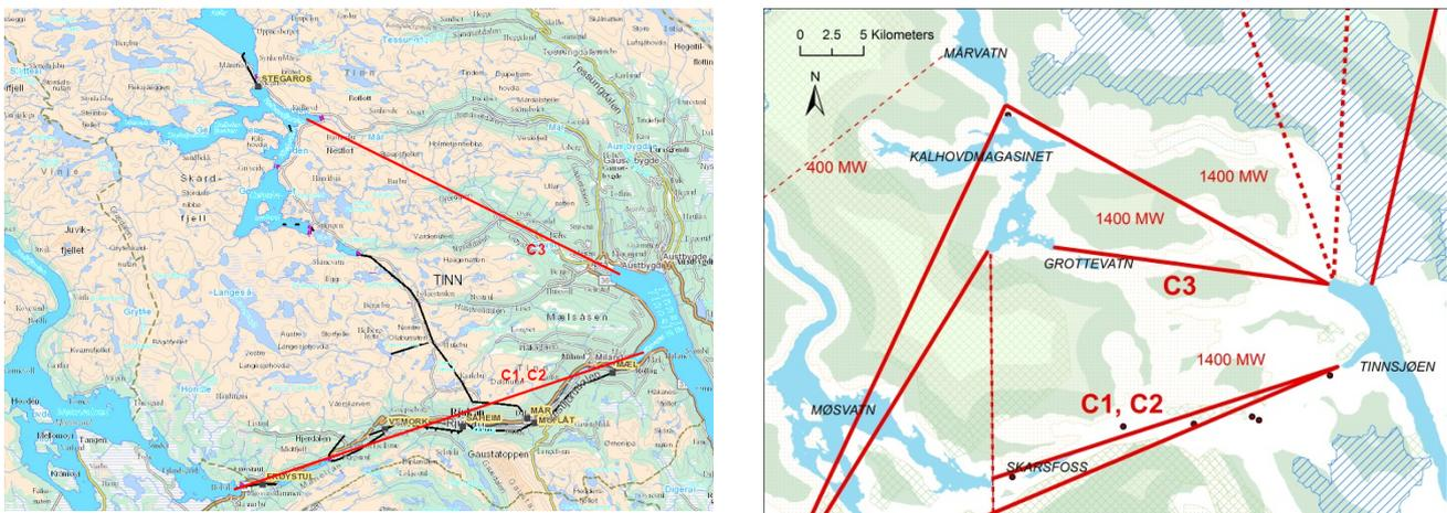
**Figure 6: The Møsvatn-Tinnsjø-Kallhovd/Mår area with the PSH cases suggested by Solvang et al. (2012, left) and the GIS-screening results obtained using the P-Mode for 400, 700 and 1400 MW. Dashed lines: PSH lines which are in conflict with the environmental restriction zones.**
