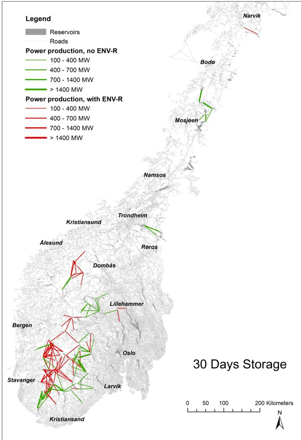
**Figure 12: PSH potential for 30 days storage duration and minimum power production of 100 MW, calculated using the T-Mode. Green lines indicate no conflicts with environmental restrictions. Red lines stand for PSH connections where these restrictions are violated.**
