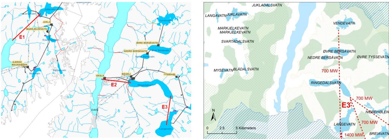
**Figure 7: Mauranger-Okslø-Tysso area with the PSH cases suggested by Solvang et al. (2012, left) and the GIS-screening results obtained using the P-Mode for 700 and 1400 MW. Dashed lines: PSH lines which are in conflict with the environmental restriction zones.**
