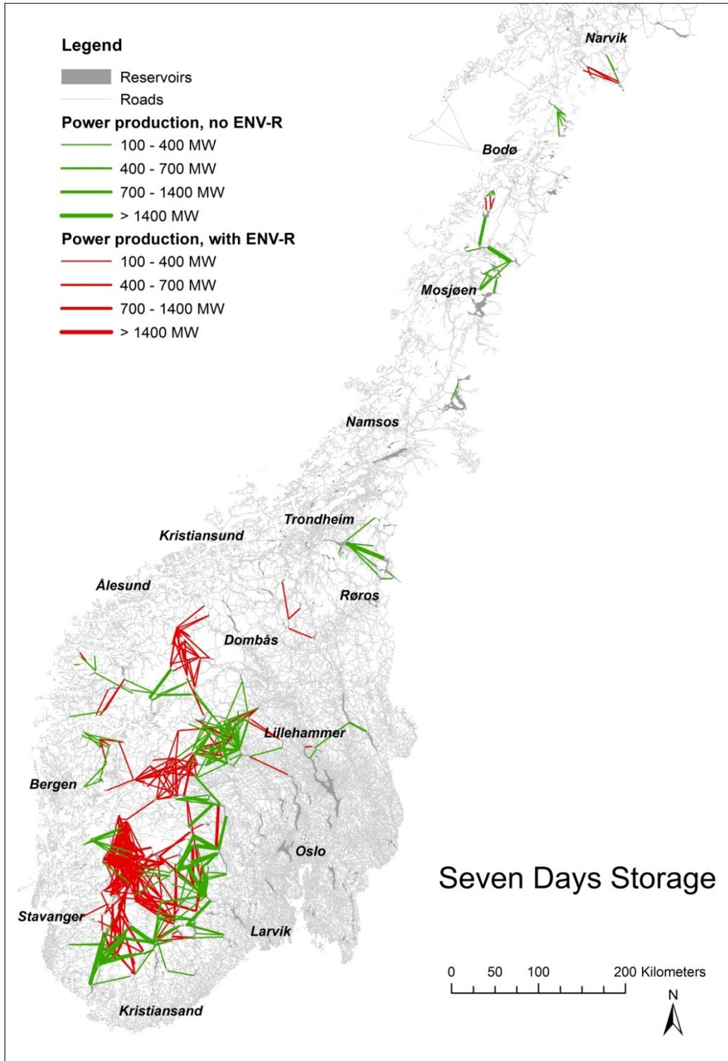
**Figure 11: PSH potential for seven days storage duration and minimum power production of 100 MW, calculated using the T-Mode. Green lines indicate no conflicts with environmental restrictions. Red lines stand for PSH connections where these restrictions are violated.**
