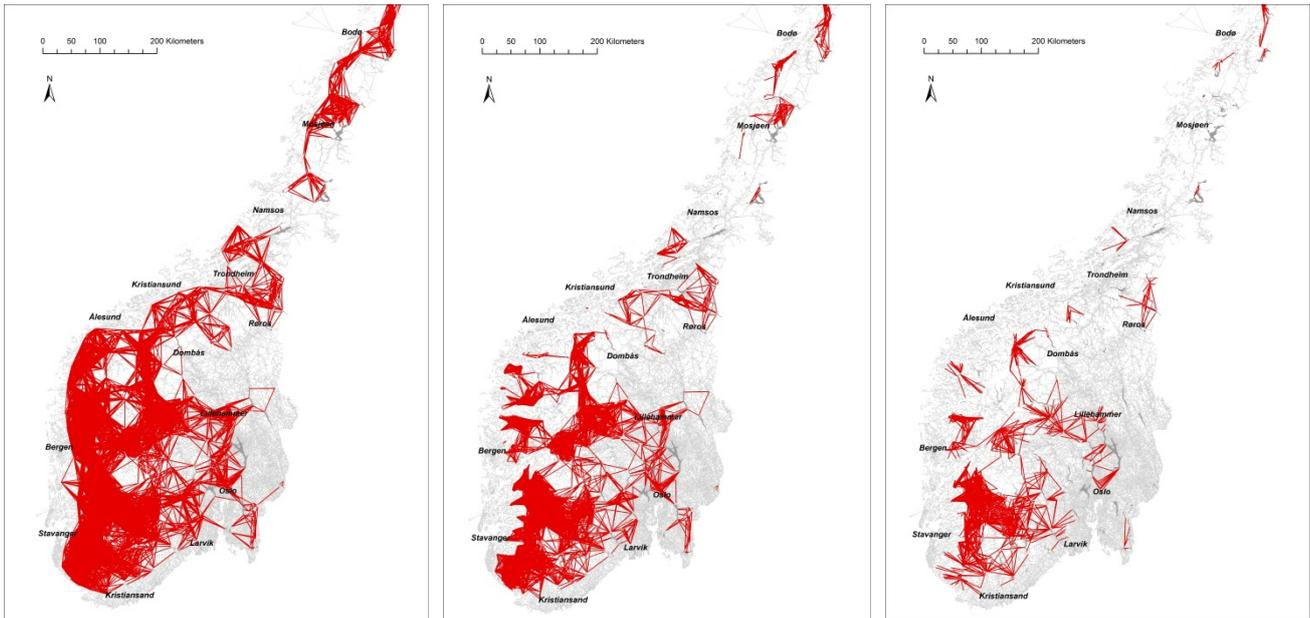
**Figure 8: PSH Lines for a maximum distance of 50 km, after application of the distance criterion (left), terrain criterion (middle), and power plant criterion (right).**
