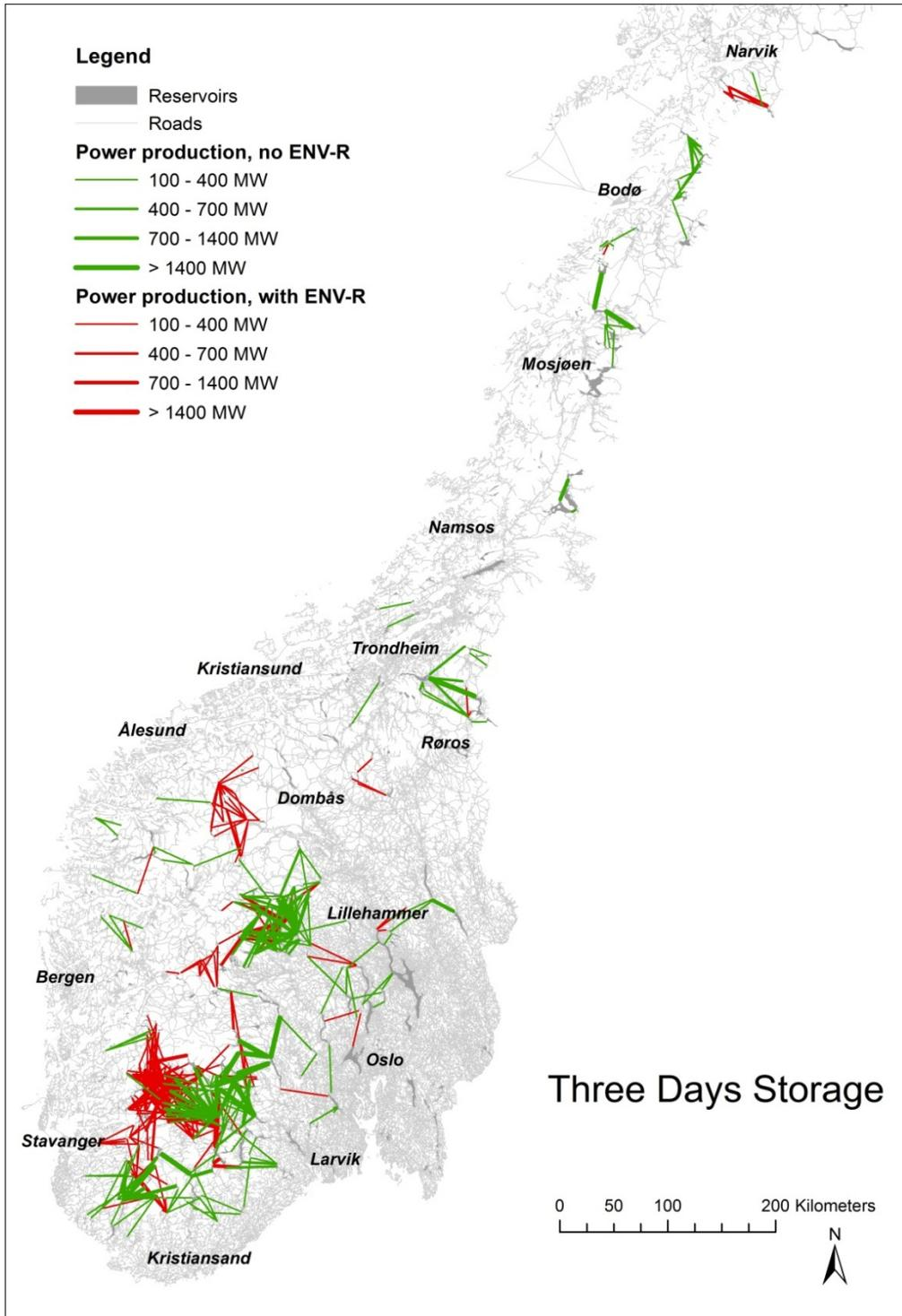
**Figure 10: PSH potential for three days storage duration and minimum power production of 100 MW, calculated using the T-Mode. Green lines indicate no conflicts with environmental restrictions. Red lines stand for PSH connections where these restrictions are violated.**
