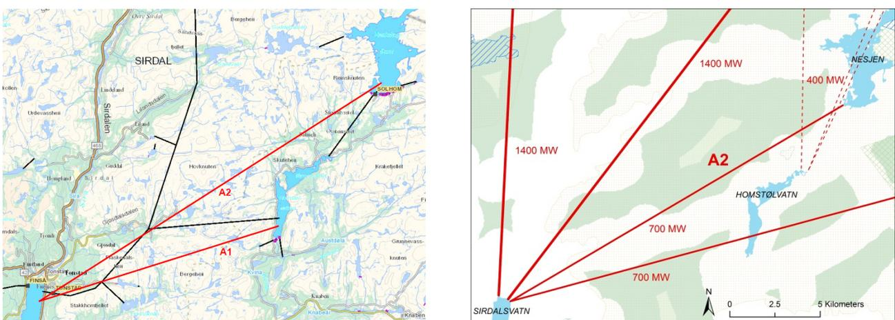
**Figure 5: The Tonstad Case from Solvang et al. (2012, left) and results of the GIS-screening for 400, 700 and 1400 MW (P-Mode). Dashed lines: PSH lines which are in conflict with the environmental restriction zones.**
