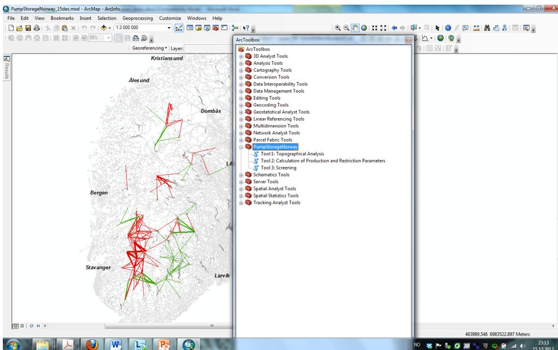
**Figure A3.1: ArcToolbox with the PumpStorageNorway script tools.**
