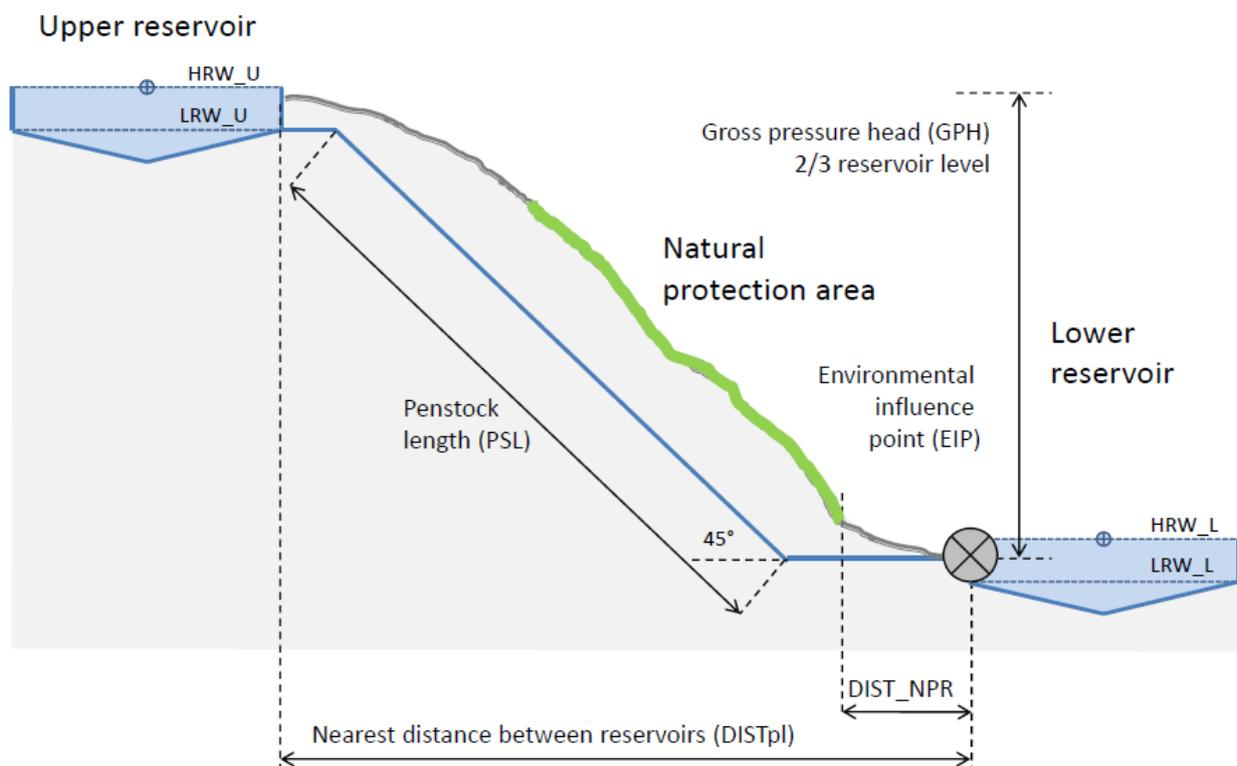
**Figure 2: Scheme of the reservoir connection with tunnel and penstock**
