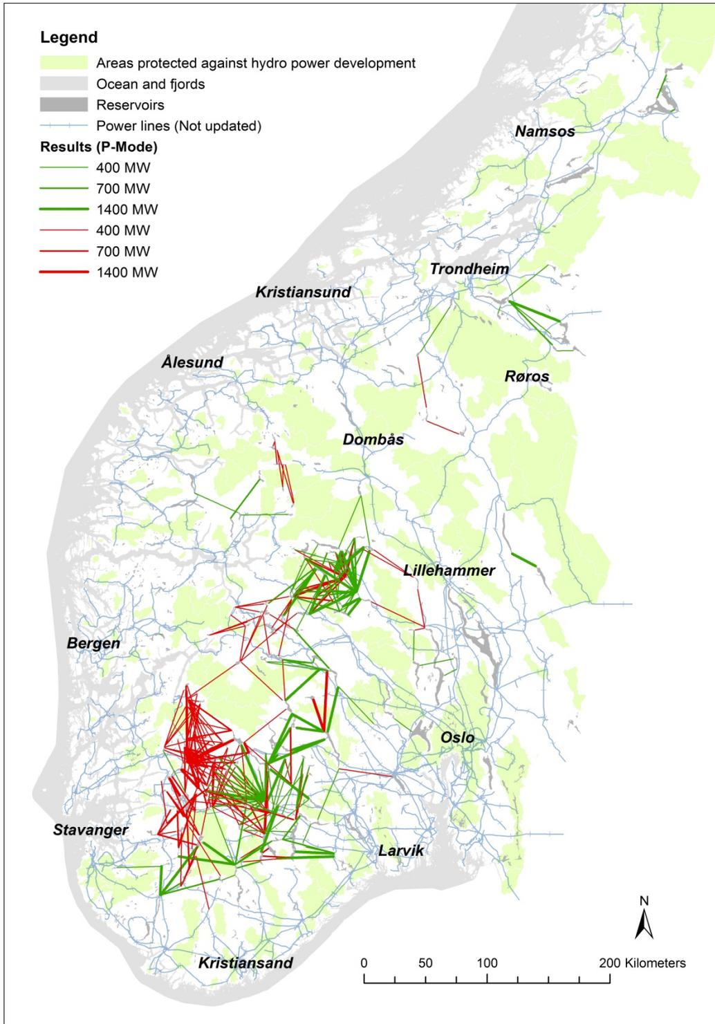
**Figure 9: PSH potential for power production of 400, 700 and 1400 MW and minimum storage duration of one day, calculated using the P-Mode. Green lines indicate no conflicts with environmental restrictions. Red lines stand for PSH connections where these restrictions are violated.**
